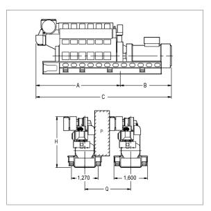
P: Free passage between the engines, width 600 mm and height 2,000 mm
