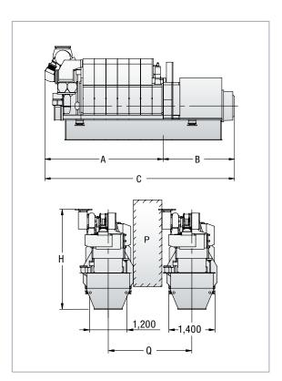
P: Free passage between the engines, width 600 mm and height 2,000 mm
